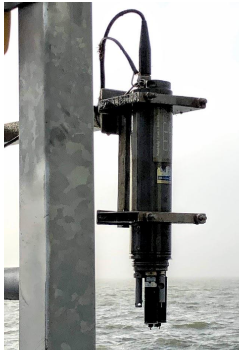
Figure 12 Multi Parameter Probe at FL67. Photo: Vincent Vuik
